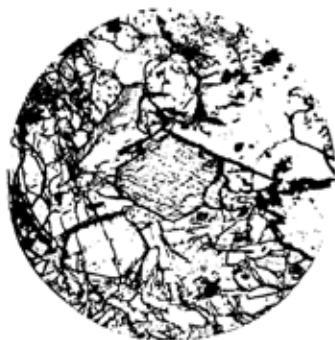
4. Glaucophane, trans. sect. Showing form and cleavages.
